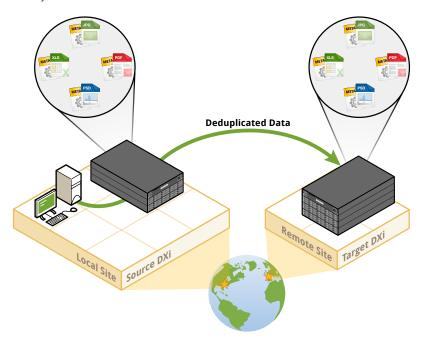
In the event of a disaster in which data on a source DXi system is lost, you can quickly *recover* the replicated data on the remote target system, allowing your business to resume normal operations.
