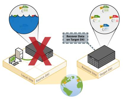
After the source DXi is back in operation at its original location, you can *fail back* data from the target DXi to the source DXi, which restores all data on the source.
