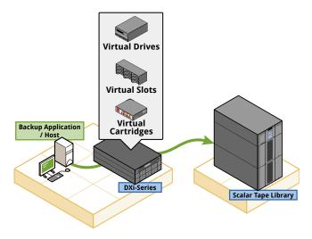
In Backup Application Specific PTT, the physical tapes contain a copy of the data from the disk copy, but they do not hold images of the virtual cartridges. This means that the virtual cartridges and physical cartridges will have different barcodes, and that they could differ in media type and cartridge count (for example, data held on one virtual DLT cartridge might be written to two physical LTO cartridges). The backup application tracks the data in both locations across the different media.
